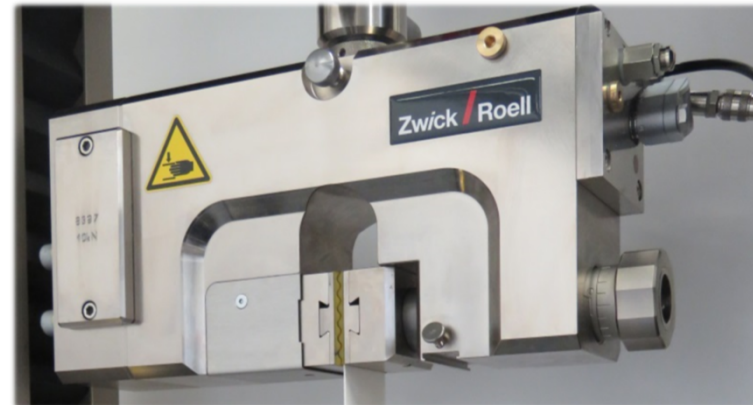
Pneumatic grip 10kN Gripping force at 6 bar → 18kN !
